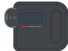
**First light red:** BGM disconnected from cellular case — try re-inserting the BGM
