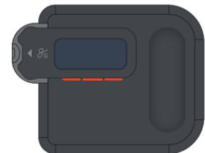
**Three red lights:** Batteries in cellular case running low — insert 3 new AAA batteries
